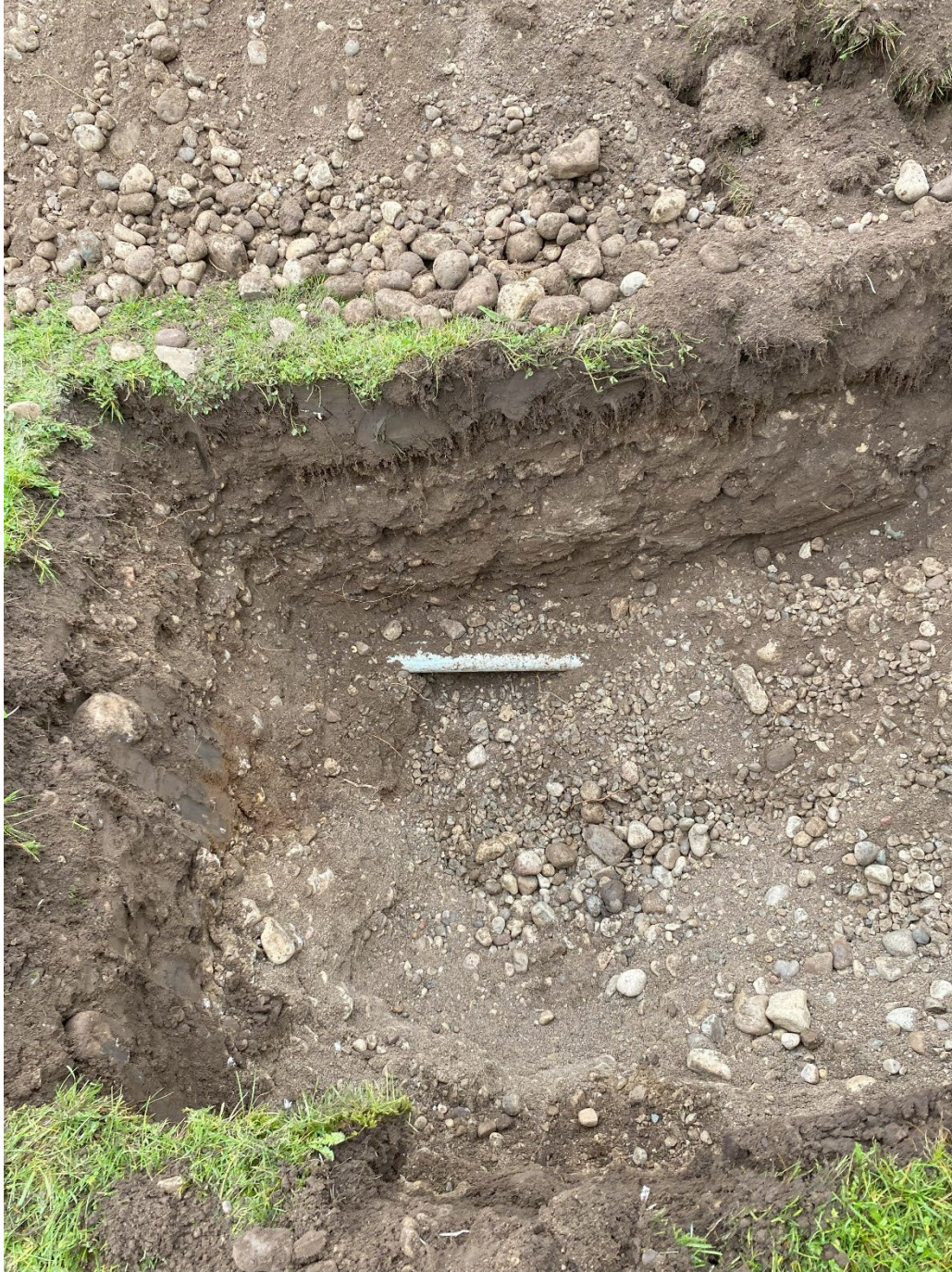
2 – Septic distribution pipe and native sand and gravel soil.
