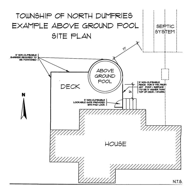
Note: This drawing is missing property lines, property lines must be on Site Plans.
