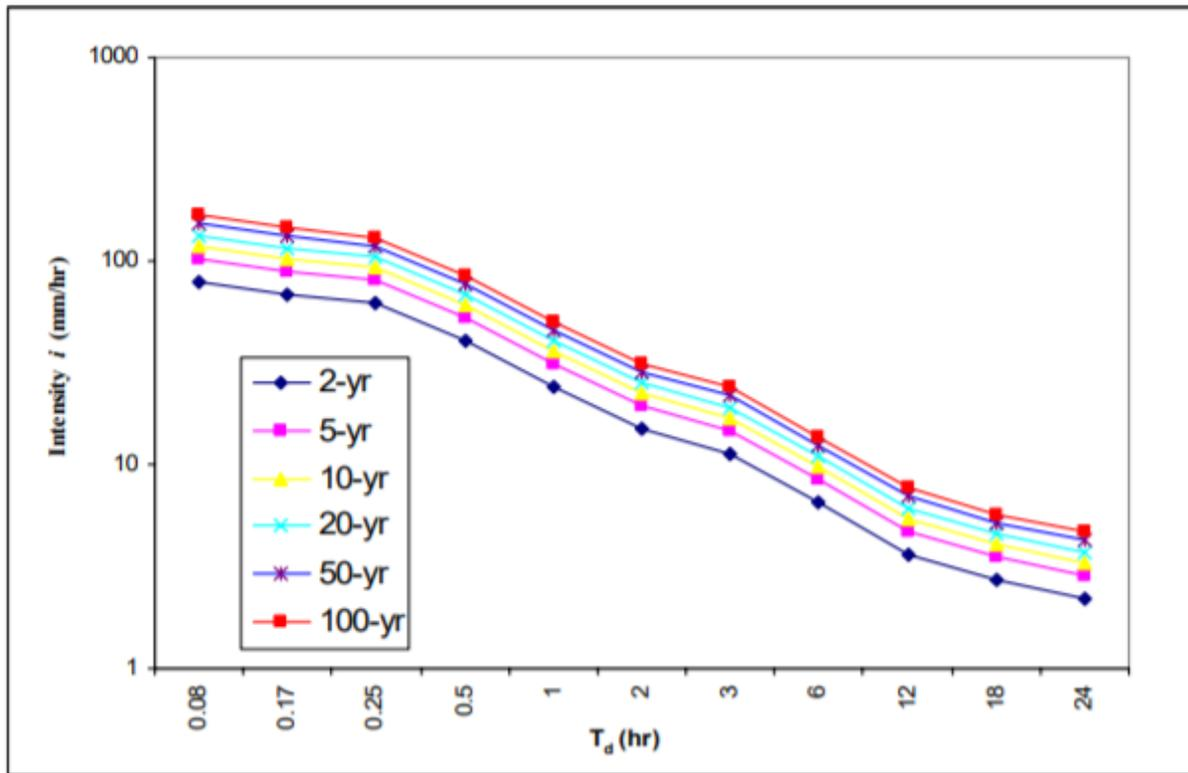
**Figure A10 – IDF Curves for Observed  $T_d$  Precipitation (1981-2000) at Station G6140954**
