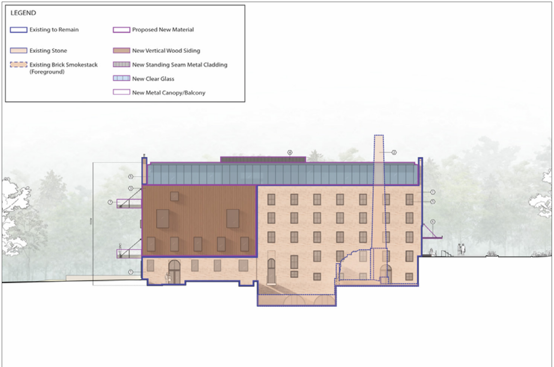
Figure 19. Facade Design and Articulation
